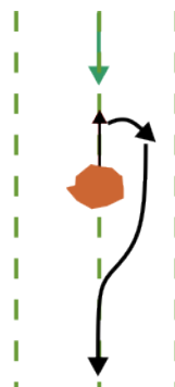
Figure 27: Manoeuvres to avoid a small obstacle in pattern mowing
