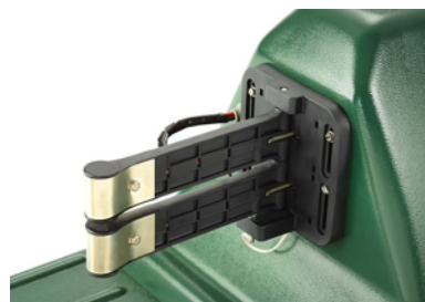
Charge contacts on the station
